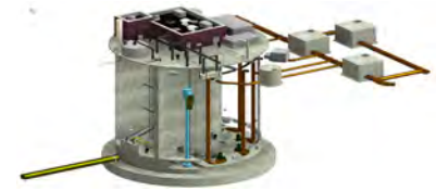
New Main Pump Station BIM 360 3D Design
