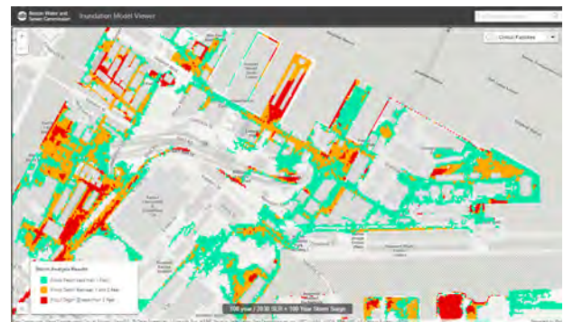
Example 2D Street Flooding Hydraulic Model
