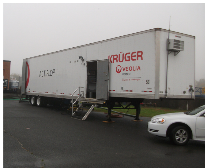
In Pittsfield, Kleinfelder led the pilot-testing for ballasted flocculation technologies including Actiflo and Comag, which eventually led to a new 40-mgd Comag tertiary treatment system.
